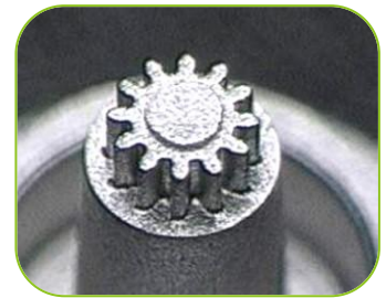
Sun gear: \phi 0.85 mm
