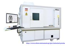
Nikon's MCT225 CT scanner is utilized in our evaluation. Unlike an optical measuring machine, there is no influence from surface reflection. Therefore, pretreatment such as surface coating is not required. In addition, it can be used to measure internal gears because it is possible to obtain non-destructive numerical data on the internal structure from the characteristics of X-ray.
