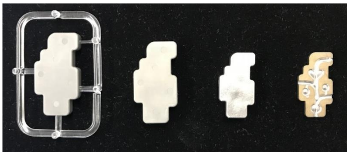
Moulding part Degassed part Sintered part Cross section
