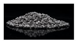
MIM material, feedstock is a mixture of metal powder and binder, which is made of plastic and wax. The binder will be completely decomposed during the process.
